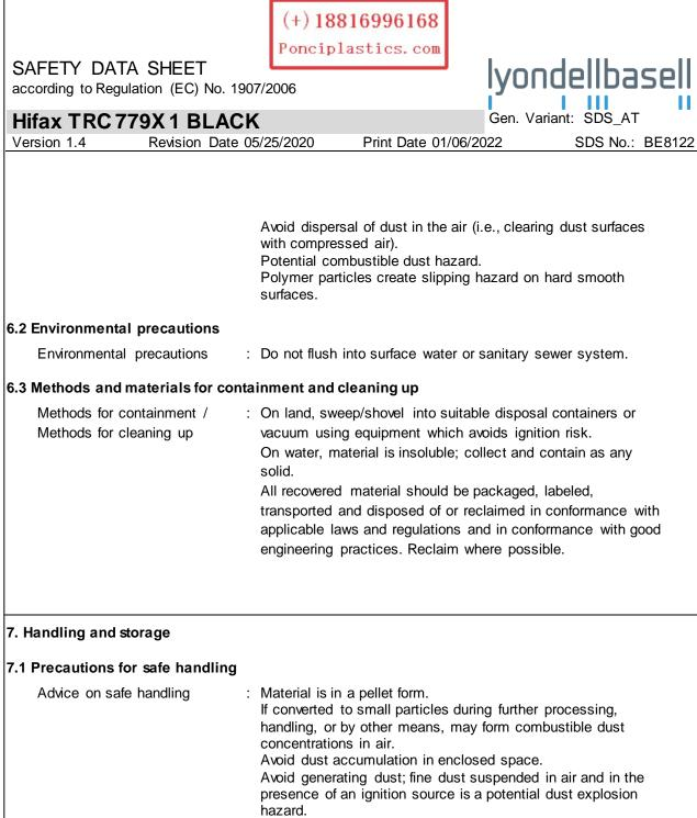
nazaro. Static discharge (spark), or other ignition sources, in high dust environments may ignite the dust and result in a dust explosion
